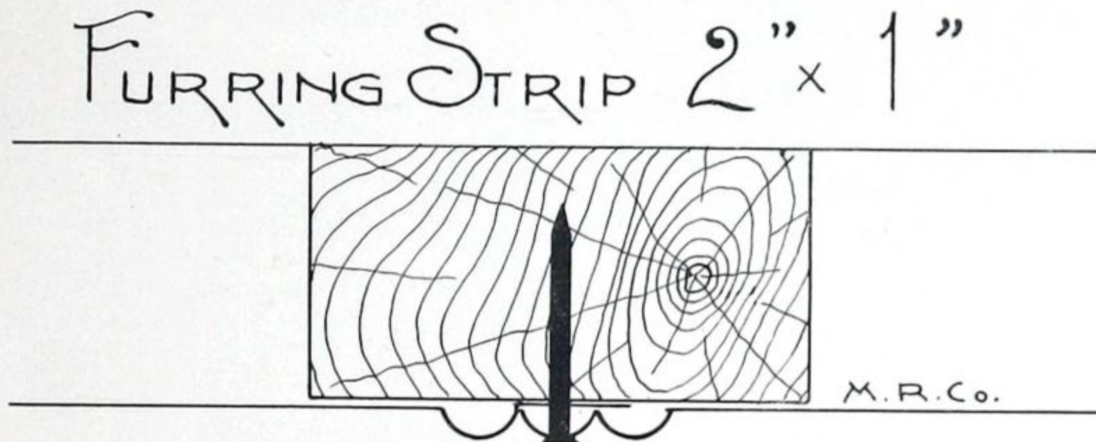
Fig. 3407.—Section of Joint on Plates Nos. 416 and 422.
